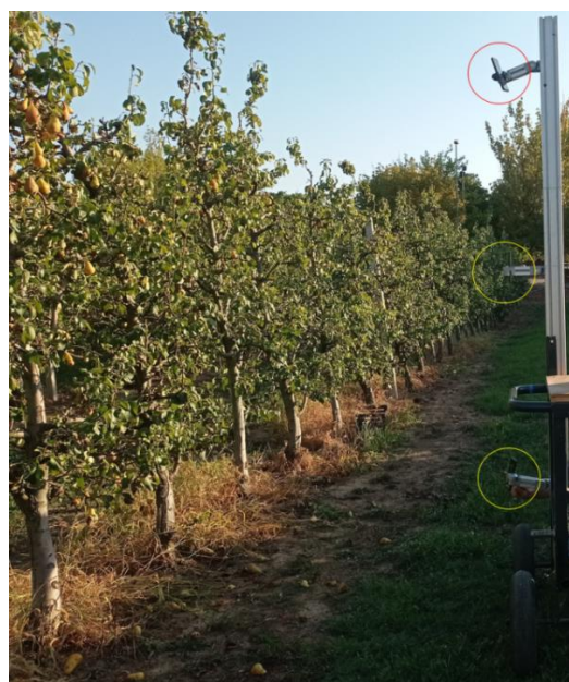
Figure. 1. Vertical structure with 3 mobile phones (highlighted with circles) at different heights.
